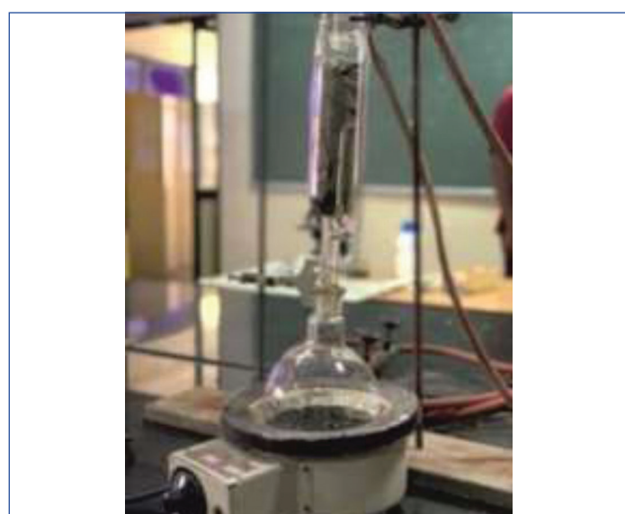
[Table/Fig-1]: Soxhlet extractor used for the preparation of methanolic extract of Plectranthus Amboinicus (PAM).
